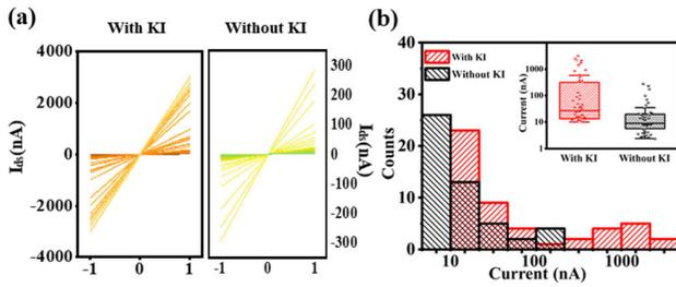
Fig. 4. (a)  $I$ - $V$  curves treated with and without KI for 50 devices. (b) Current statistics of the device fabricated with and without KI.
