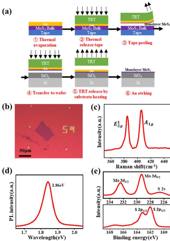
Fig. 1. (a) Device process for the gold-assisted exfoliation to fabricate monolayer MoS<sub>2</sub>. TRT is short for thermal release tap. (b) Optical image of the monolayer MoS<sub>2</sub>. (c) Photoluminescence spectrum of MoS<sub>2</sub> under green laser excitation ( $\lambda = 532$  nm). (d) Raman spectroscopy of MoS<sub>2</sub>. (e) XPS of Mo 3d (top panel) and S 2p (bottom panel) spectra for MoS<sub>2</sub>.
