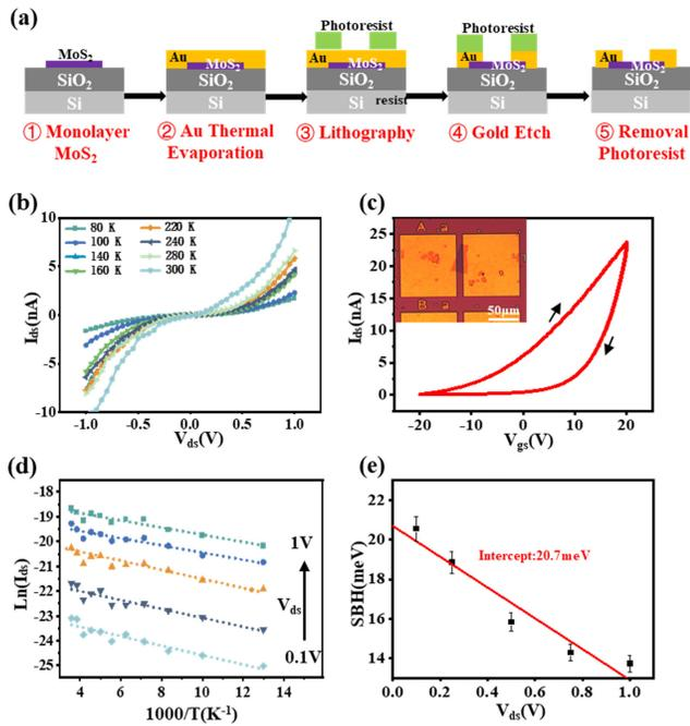
**Fig. 2.** (a) Fabrication process for MoS<sub>2</sub> devices with pure gold electrode contact. (b)  $I$ - $V$  curves at different temperatures. (c) Gate transfer characteristics of the MoS<sub>2</sub> transistor (inset: device optical microscopic image). (d) Linear fit of  $\ln(I_{ds})$  versus  $1000/T$ . (e) Slopes extracted from the linear fit is plotted as a function of  $V_{ds}$  and  $\Phi_B$  is derived from its  $y$ -intercept.
