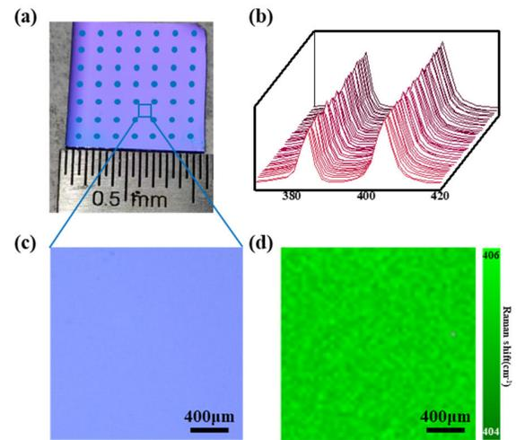
Fig. 5. (a) MoS<sub>2</sub> monolayer synthesized on a SiO<sub>2</sub>/Si substrate. The marked dots are where Raman spectra are taken. (b) Raman mapping spectra from different locations marked in (a). (c) Optical microscope image of a 2 mm region arbitrarily selected from the sample. (d) Raman mapping of the A<sub>1g</sub> peak of MoS<sub>2</sub> within the region shown in (c).
